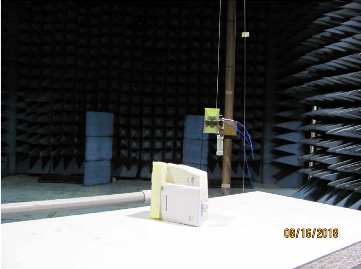
The EUT was taped to a foam stand in order to change the axis of rotation.
