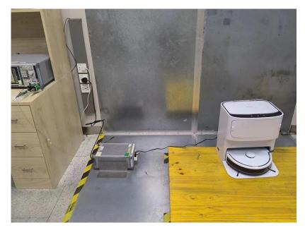
Radiated Emissions From 30MHz-1000MHz
