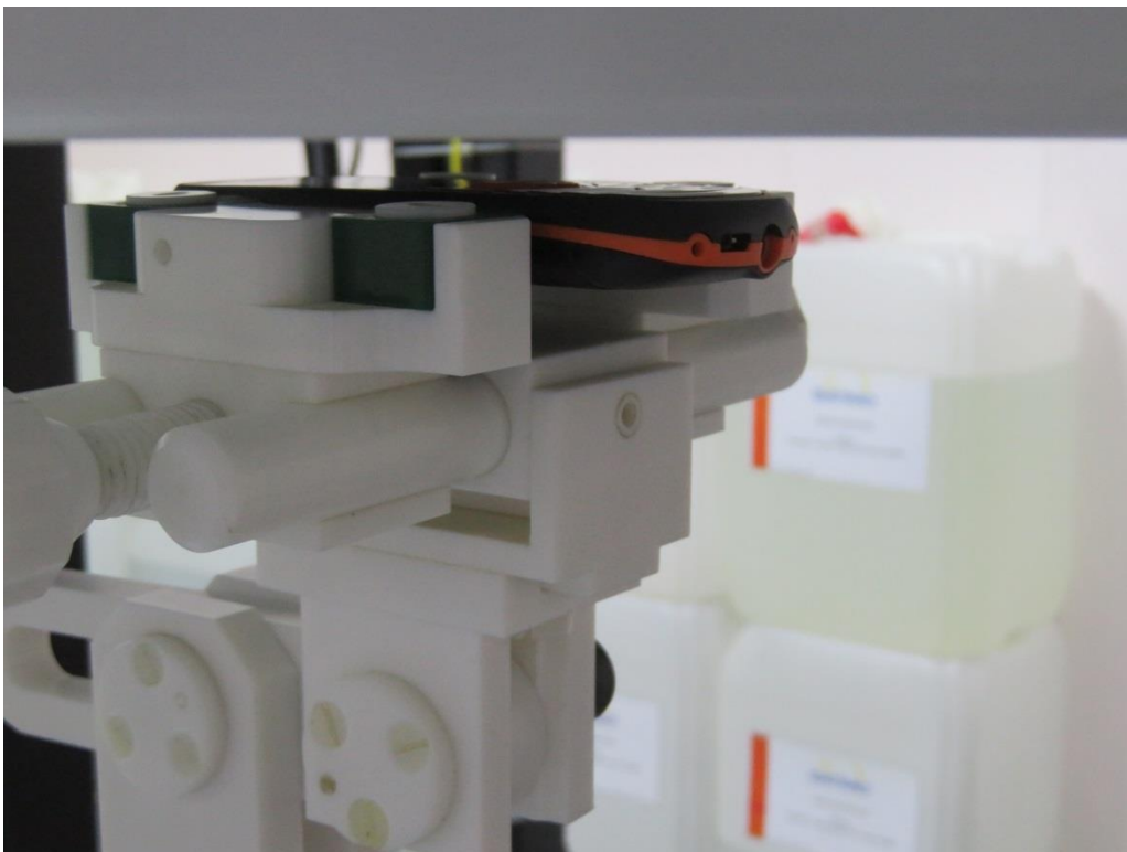
10mm body-worn Front Side Setup Photo
