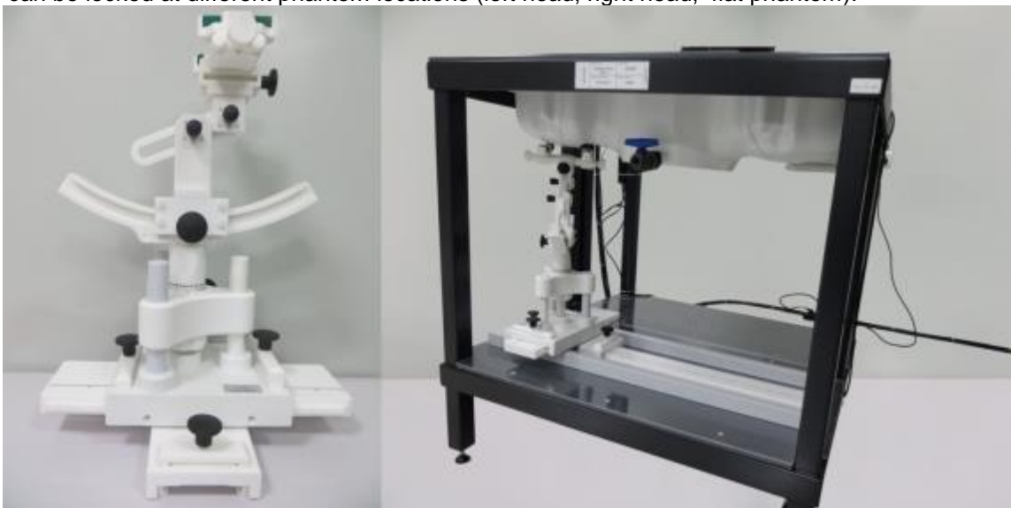
Device holder supplied by SATIMO
