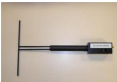
Figure 1 – Satimo COMOSAR Validation Dipole
