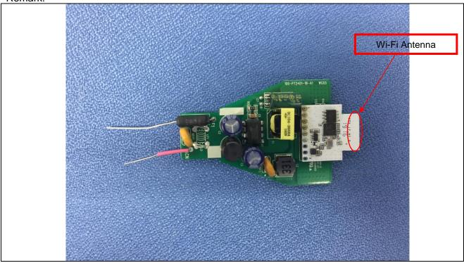
Details of: Driver PCB rear view
