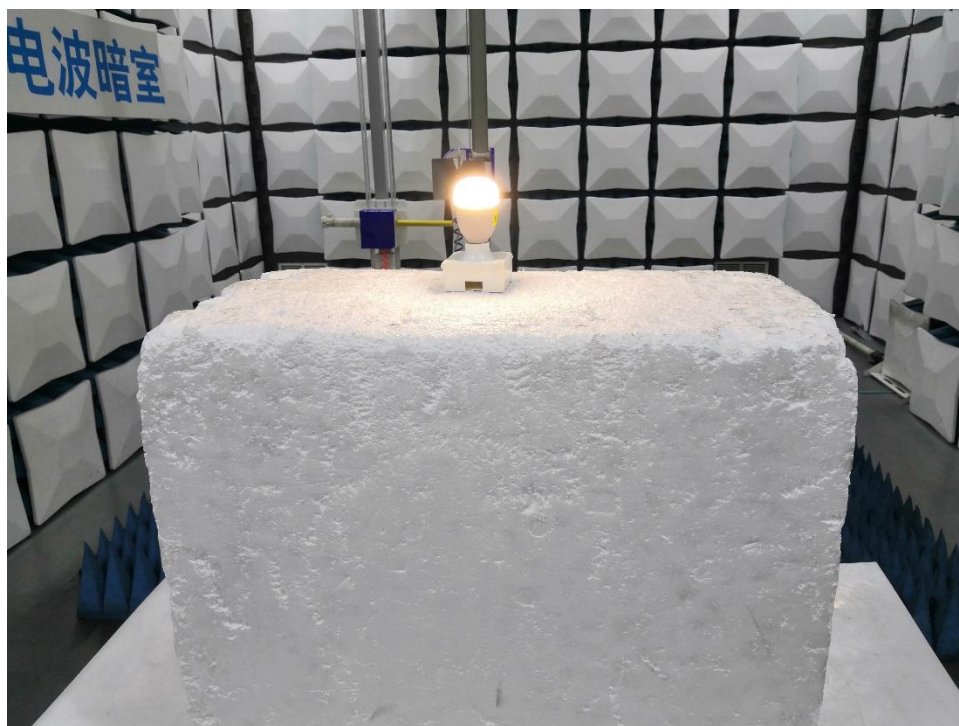
Radiated Emission test Above 1GHz
