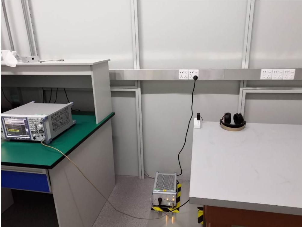
FCC RADIATED EMISSION TEST SETUP
