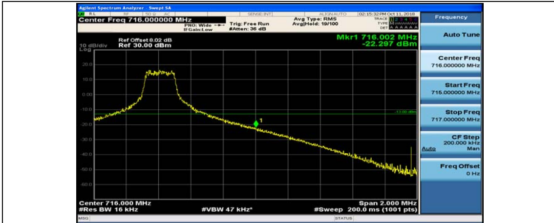
Channel Bandwidth: 10 MHz_HCH_16QAM_25RB#0
