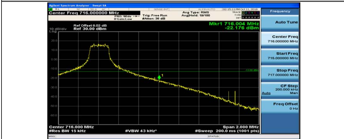
Channel Bandwidth: 10 MHz_HCH_QPSK_25RB#0
