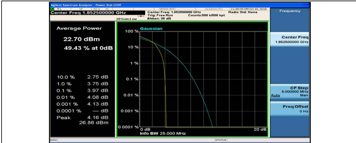
(Channel Bandwidth: 5 MHz)_LCH_16QAM_12RB#6
