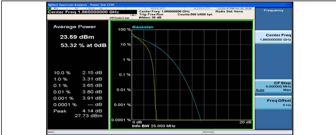
(Channel Bandwidth:20 MHz)_LCH_QPSK_50RB#25
