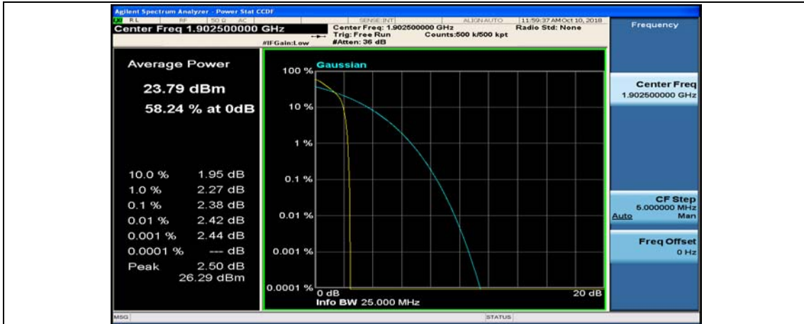
(Channel Bandwidth:15 MHz)_HCH_QPSK_1RB#74
