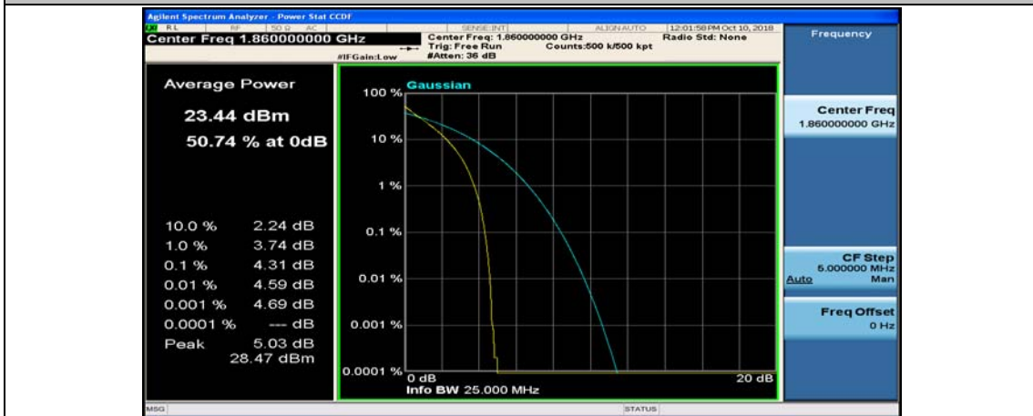
(Channel Bandwidth:20 MHz)_LCH_QPSK_100RB#0
