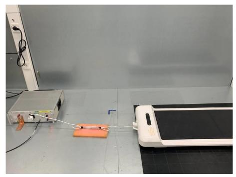
Radiated Emission test below 1GHz
