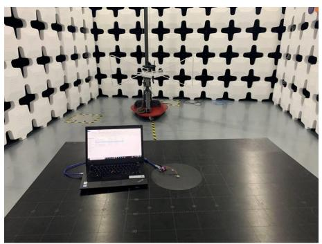
Radiated Emission test Above 1GHz
