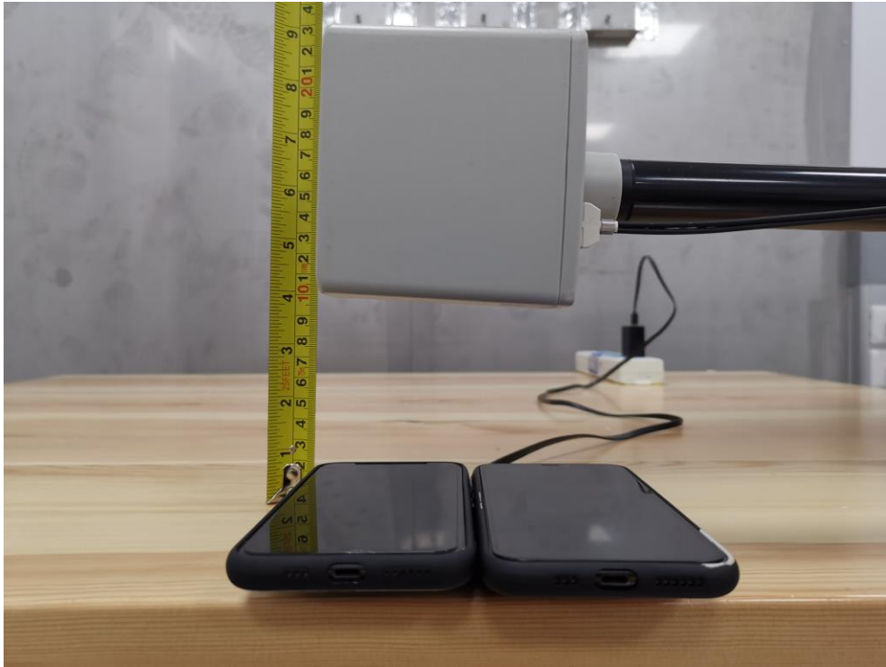
Test setup of E side with Coil 1 + Coil 2
