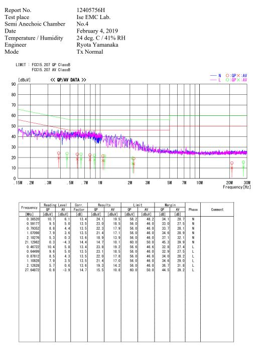
CHART: WITH FACTOR Peak hold data. CALCULATION : RESULT = READING + C.F (LISN + CABLE + ATT) Except for the above table: adequate margin data below the limits.
