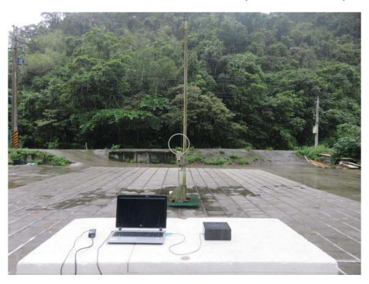
Radiated Measurement Photos (30MHz to 1GHz)
