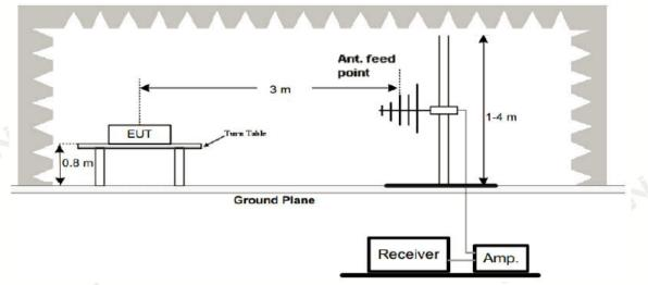
3. Radiated Emission Test-Up Frequency Above 1GHz
