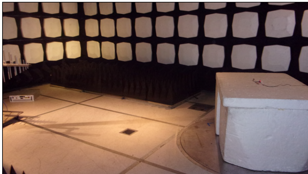
Figure 2: Radiated Emissions – 30MHz – 1GHz
