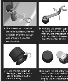
**Tips:** When installing the cover, pay attention to check whether the waterproofing is in place. If it is damaged, please replace it with a new waterproof ring and then install the casing.
