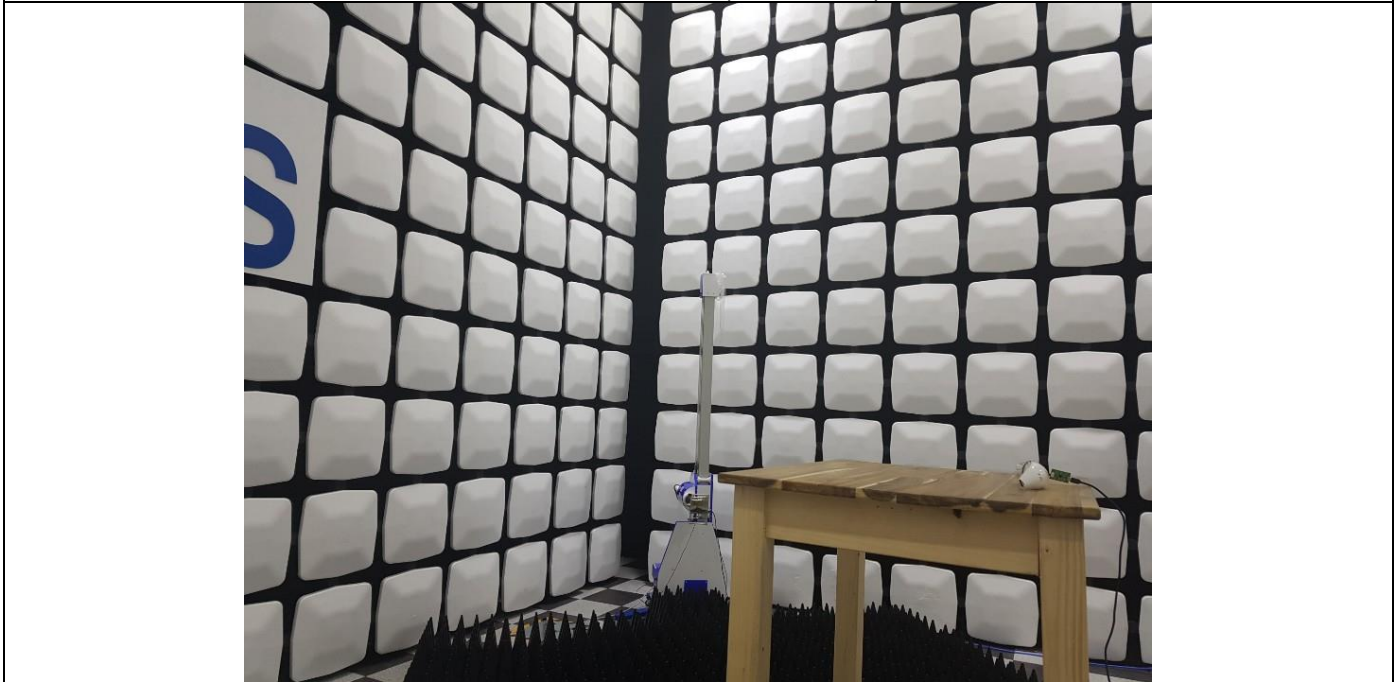
Radiated Test (Above 1G)
