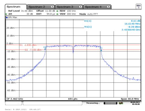
802.11n(HT20) mode with 6.5Mbps data rate Channel 1: 2.412GHz:
