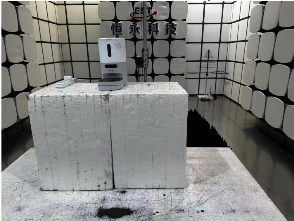
Radiated Test (Above 1GHz)
