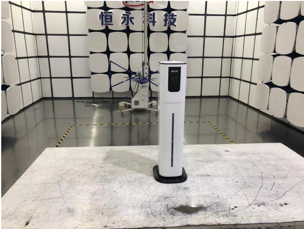
Radiated Test (30-1000 MHz)
