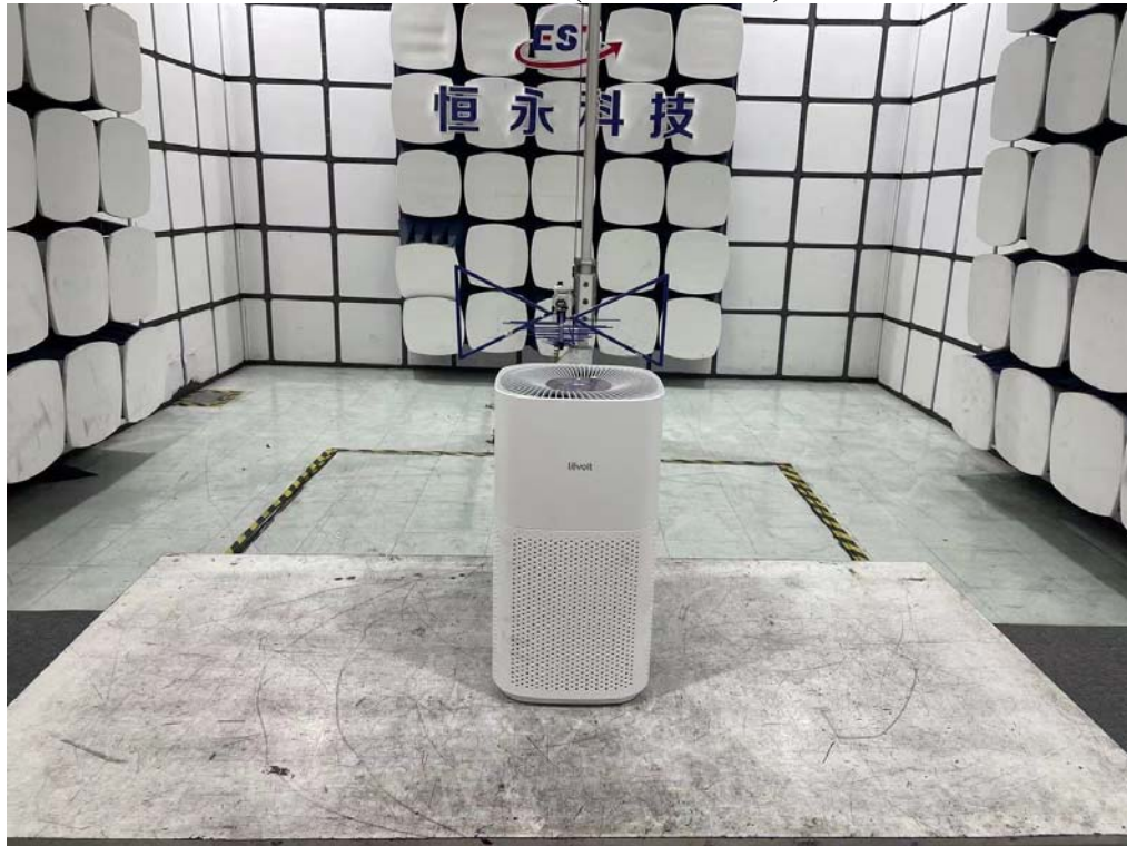
Radiated Test (Below 1GHz)
