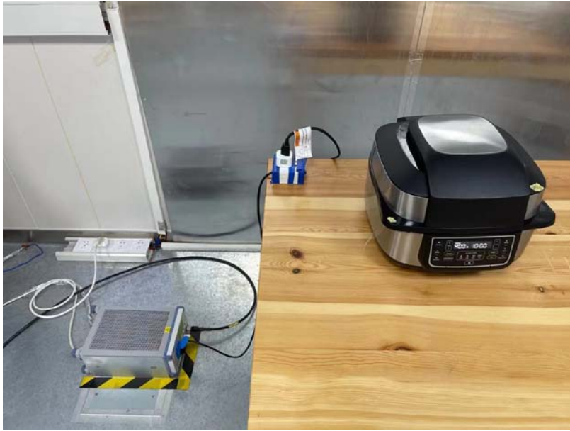
Conducted emission test setup
