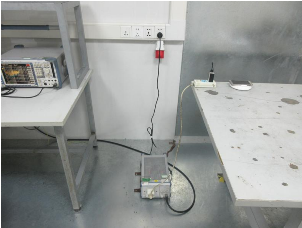
Photo of Conducted Emission Measurement
