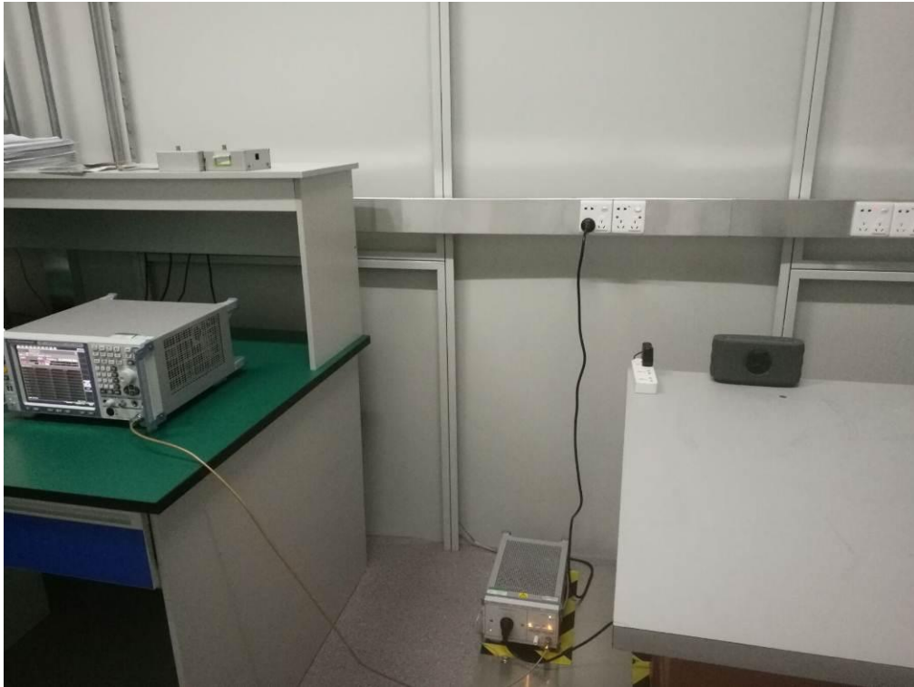
FCC RADIATED EMISSION TEST SETUP
