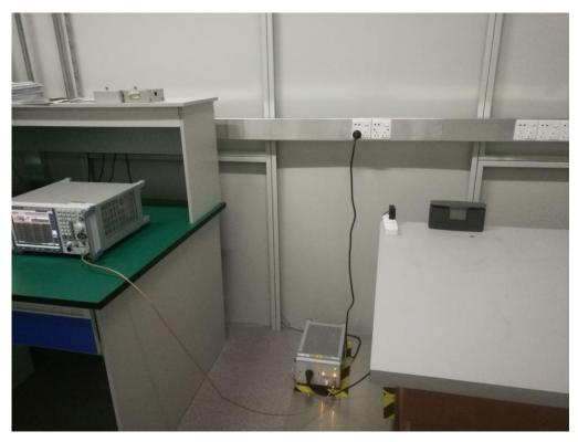
FCC RADIATED EMISSION TEST SETUP
