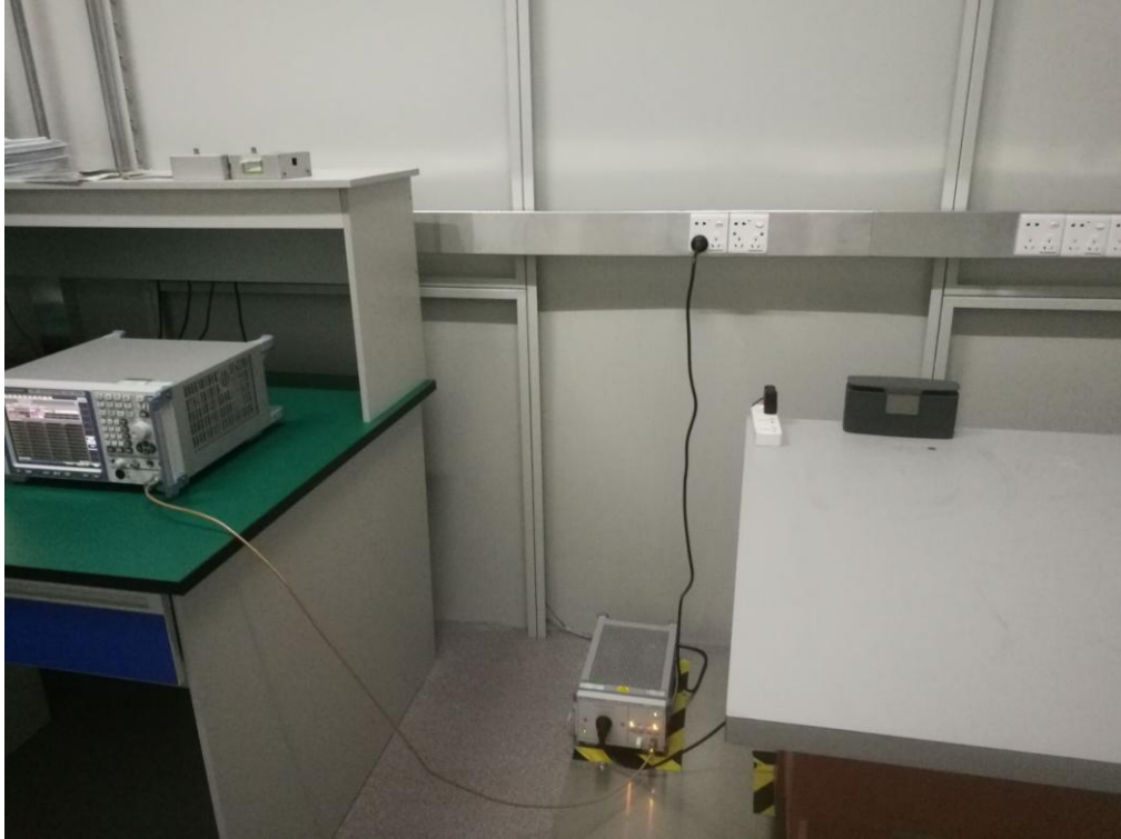
FCC RADIATED EMISSION TEST SETUP
