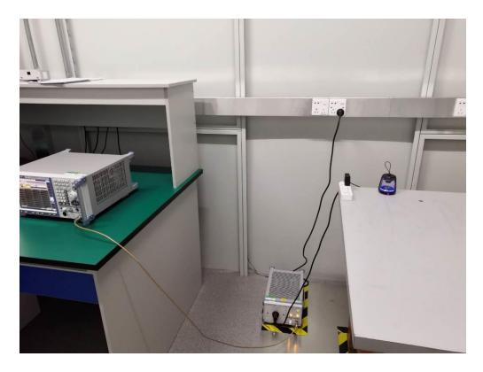
FCC RADIATED EMISSION TEST SETUP
