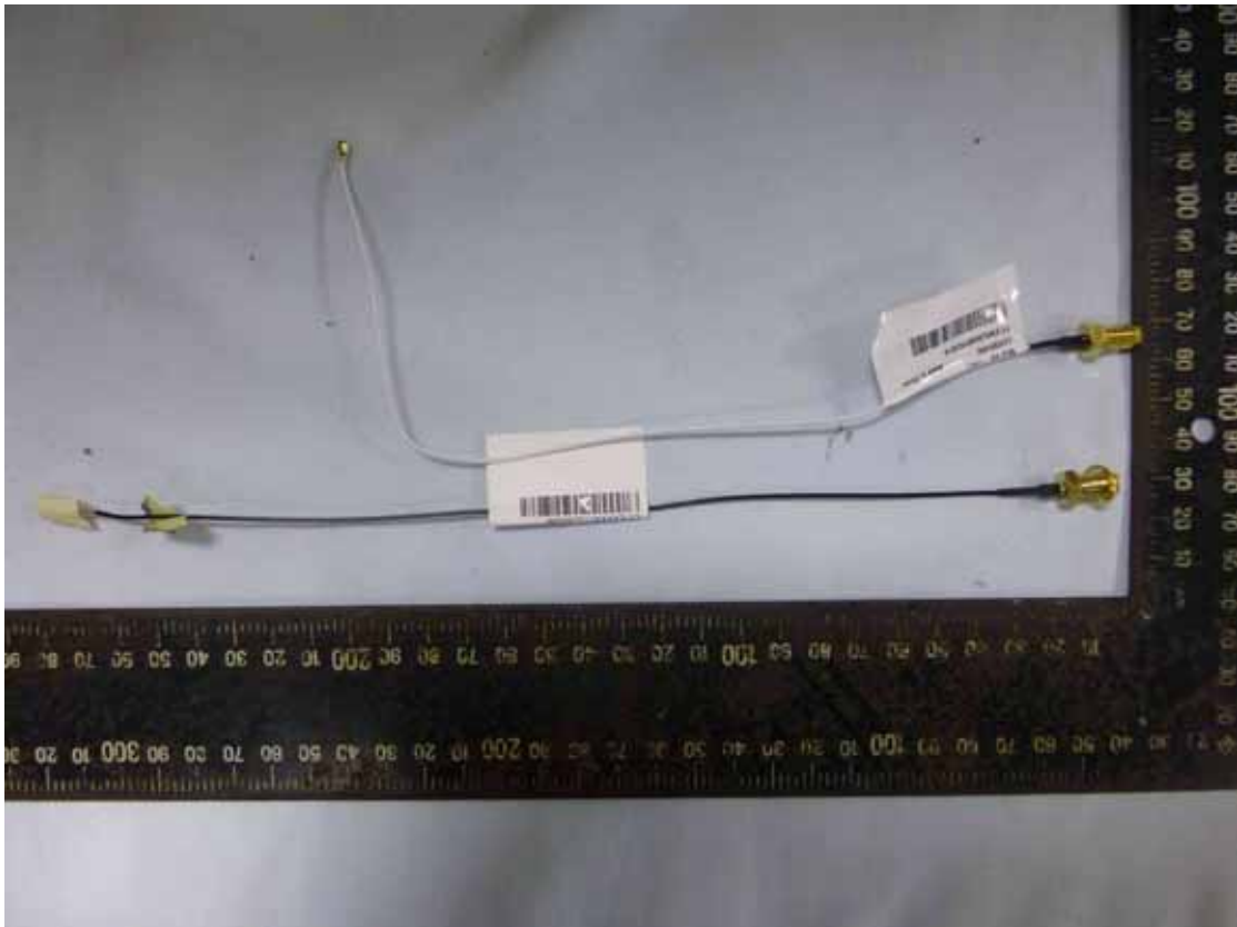
Figure 44 WIFI Cable&LTE Cable
