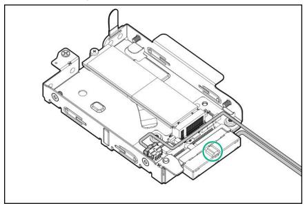
**10.** Install the stand off nut on the drive cage.
