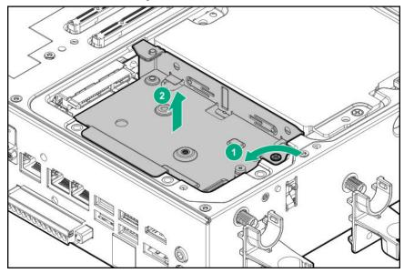
8. Install the M.2 adapter board on the drive cage.
