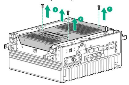
**b.** Detach the pins of the security cover from the system, and then remove the security cover.
