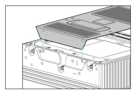
**b.** Install the screws on the security cover and secure it to the system.
