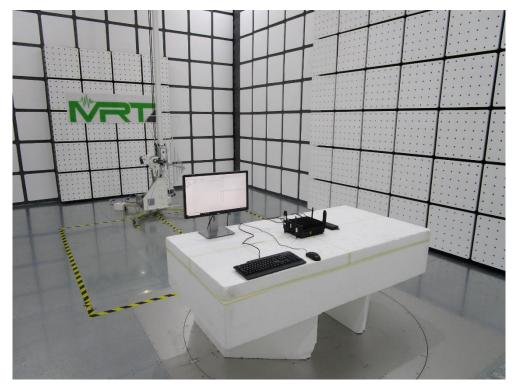
Description: Radiated Emission Test Setup for 1GHz~18GHz
