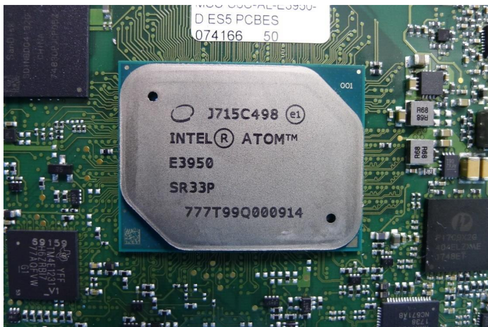
(24) CPU Board (Intel Atom E3950)
