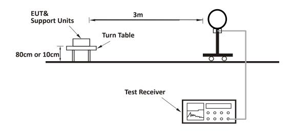
For Radiated emission 30MHz to 1GHz:
