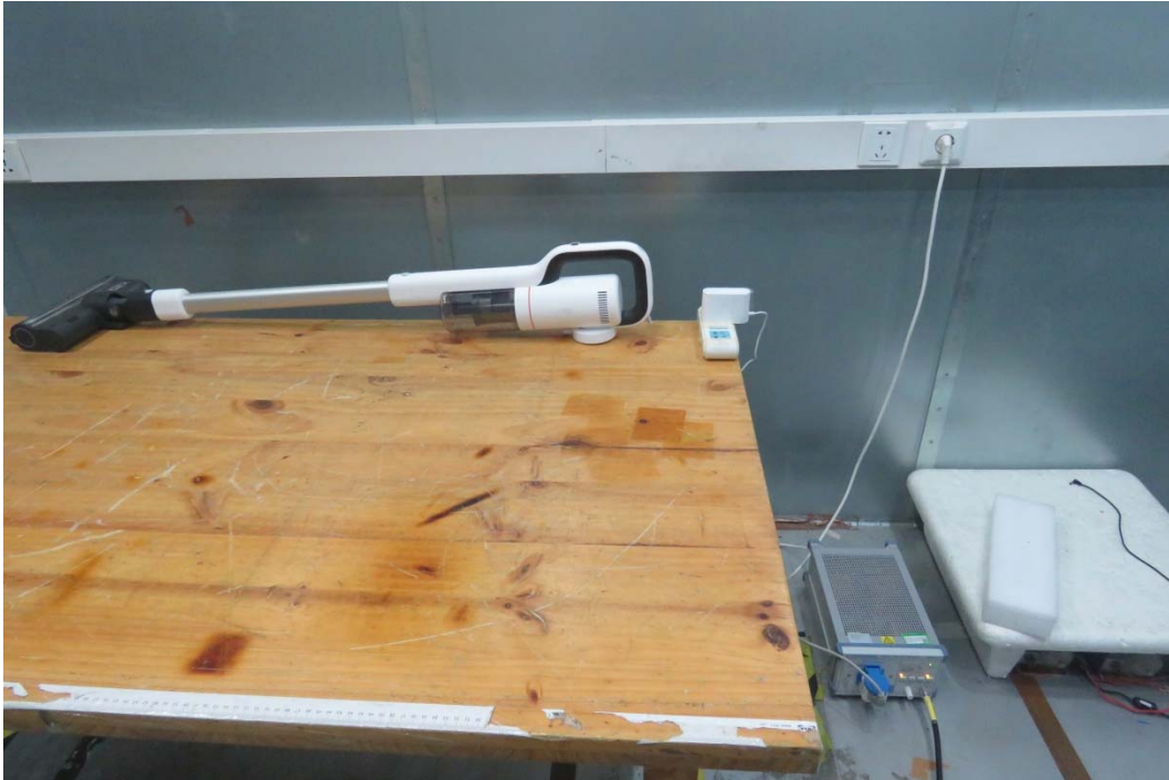
Picture 2 Conducted Emission Test Setup
