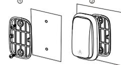
Tip: Please avoid installing on metal objects (iron gates, iron windows, etc.) to avoid affecting the launch distance. Please try it before fixed transmitter.
