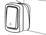
Tip: Please avoid installing on metal objects (iron gates, iron windows, etc.) to avoid affecting the launch distance. Please try it before fixed transmitter.
