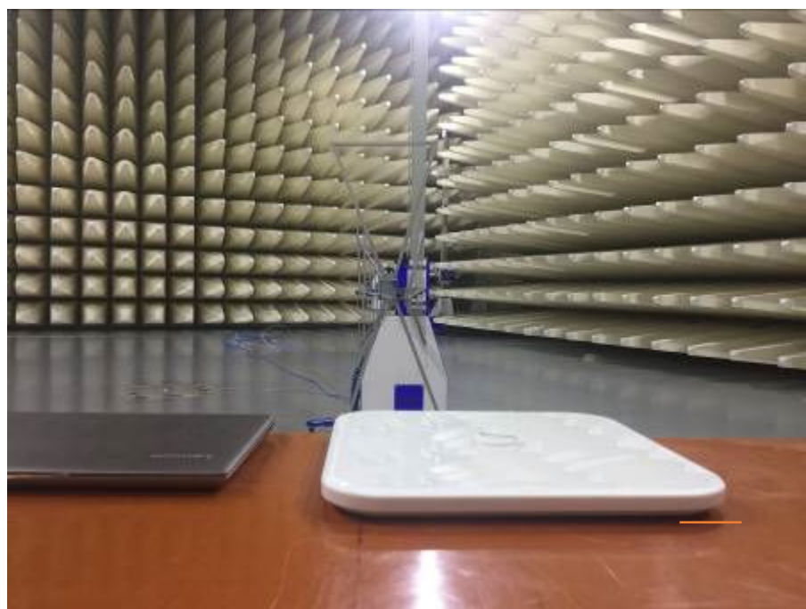
Spurious Radiated Emissions Test setup (below 1GHz)
