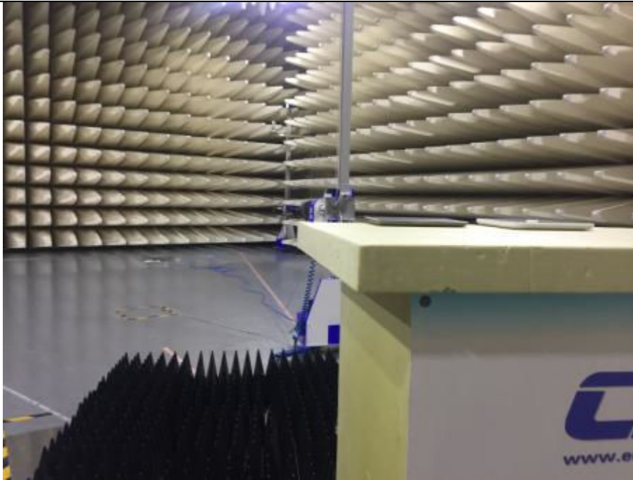
Spurious Radiated Emissions Test setup (1GHz~25GHz)
