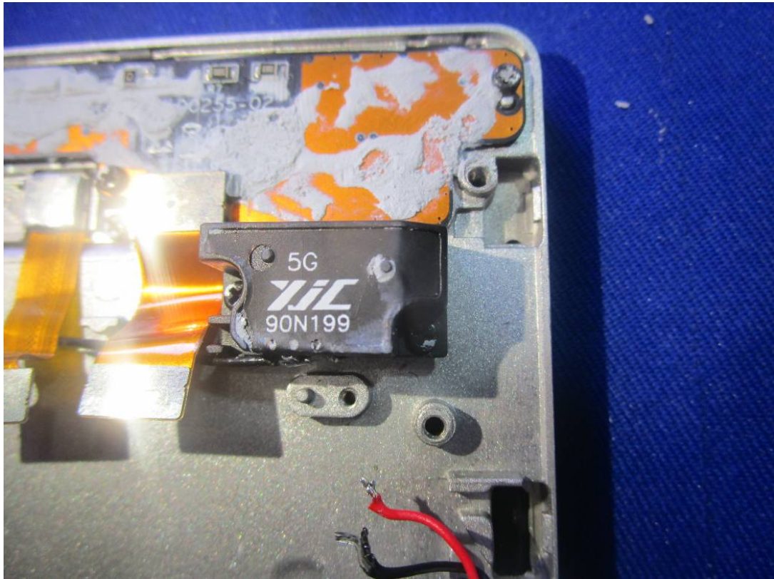
5G Antenna View
