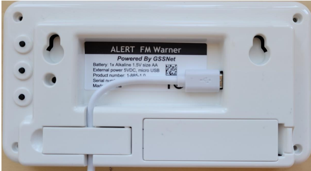
Power cable inserted
