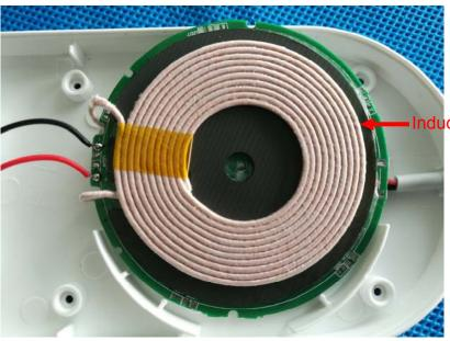
Inductive loop coil Antenna
