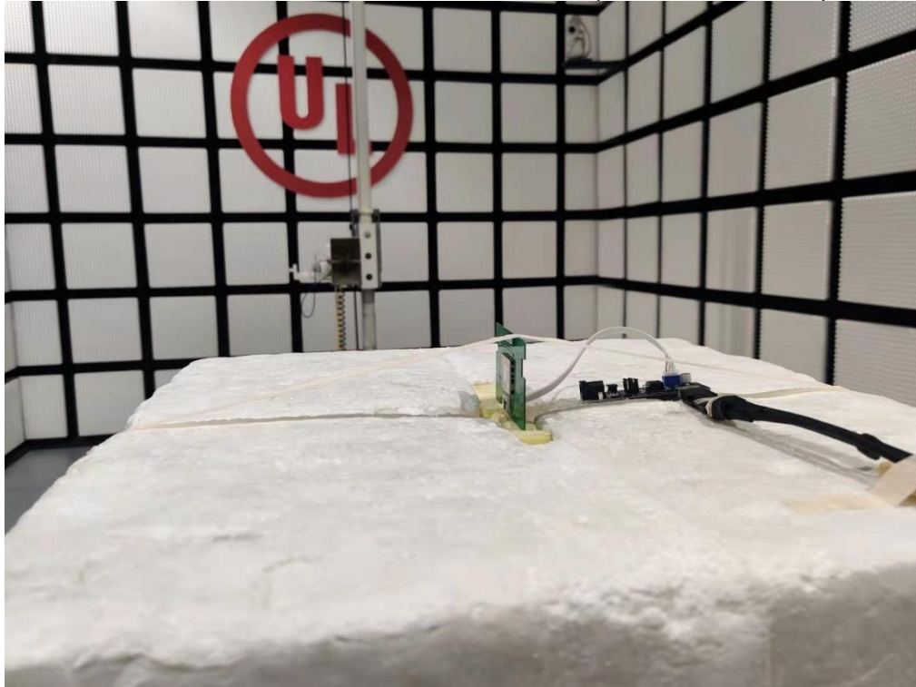
RADIATED RF MEASUREMENT SETUP (Above 1G – Y axis)
