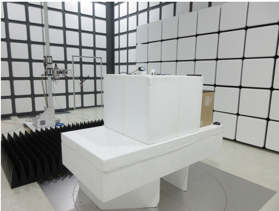
Description: Radiated Emission Test Setup for 1GHz~18GHz
