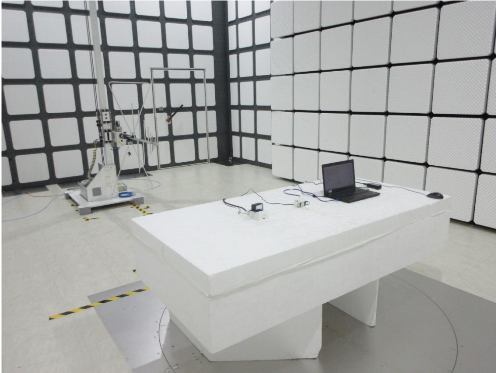
Description: Radiated Emission Test Setup for 1GHz~18GHz
