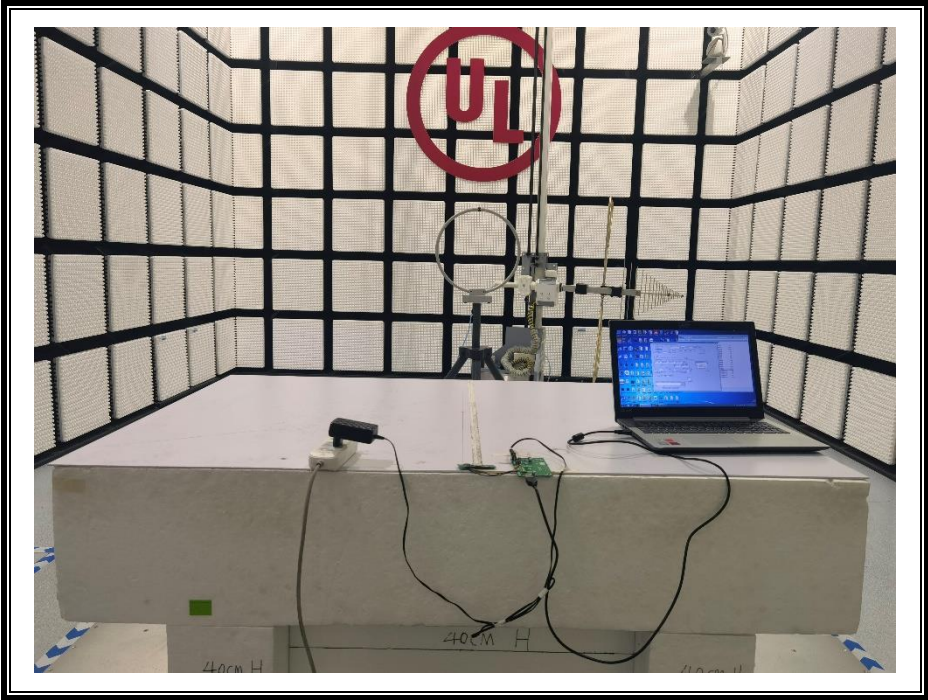
RADIATED RF MEASUREMENT SETUP for WIFI (Below 30MHz)
