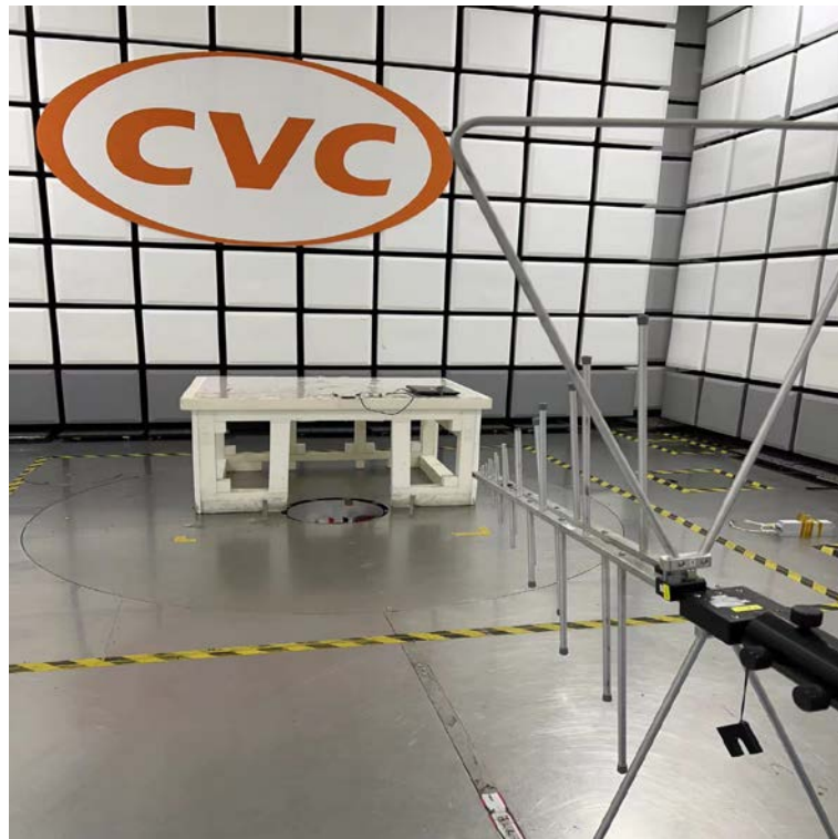
(2) Radiated spurious emission Test Setup(Below 1GHz)
