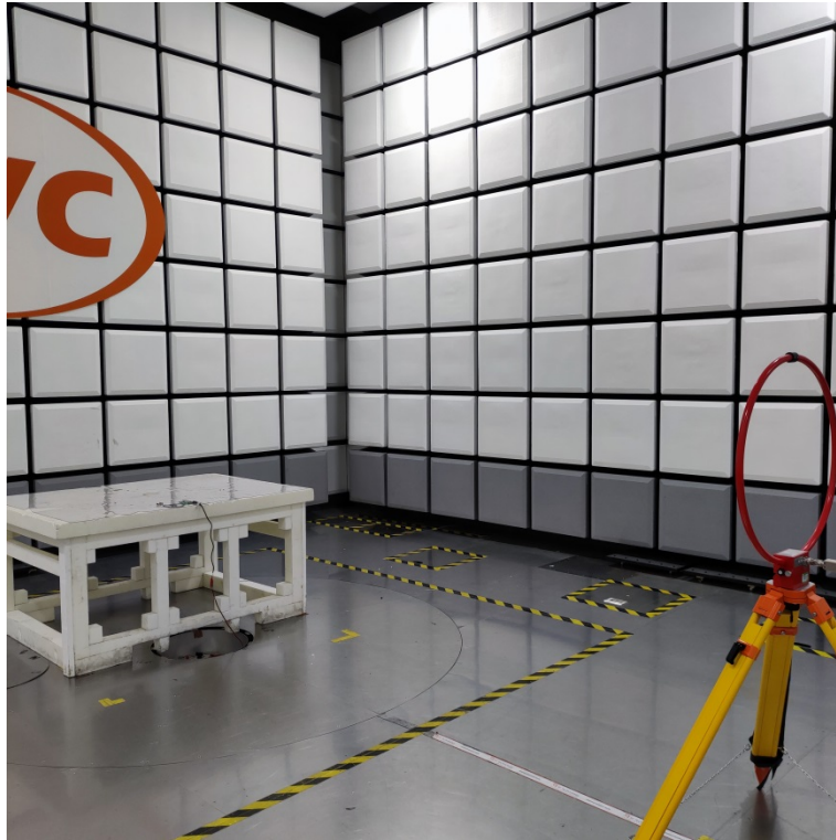
(2) Radiated spurious emission Test Setup(Below 1GHz)
