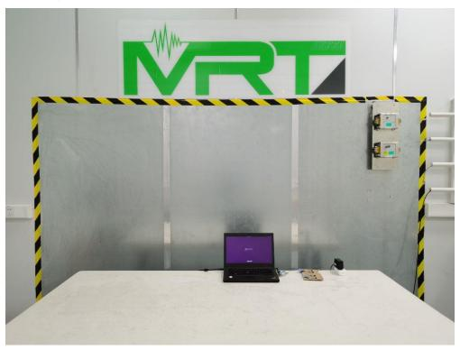
Description: Front View of Conducted Emission Test Setup for Power Port
