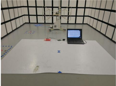
RADIATED RF MEASUREMENT SETUP (Below 30MHz)
