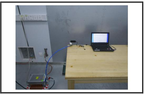
RADIATED RF MEASUREMENT SETUP (Below 1 GHz)
