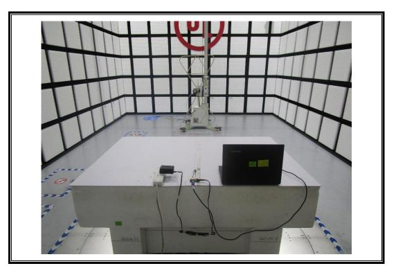
RADIATED RF MEASUREMENT SETUP (Below 30MHz)
