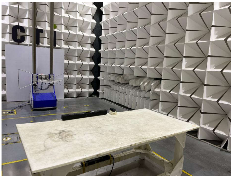
Radiated spurious emission Test Setup-1(Below 1GHz)
