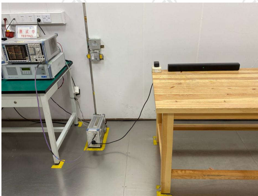
AC Power Line Conducted Emission
