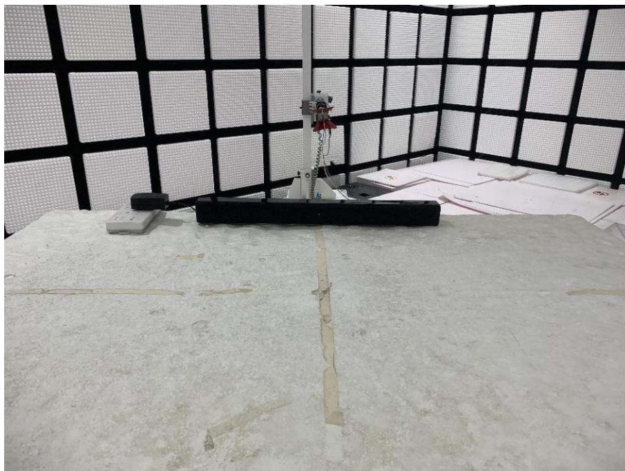
Radiated spurious emission Test Setup-2(Above 1GHz)
