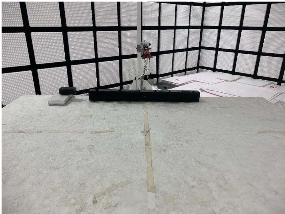
Radiated spurious emission Test Setup-2(Above 1GHz)
