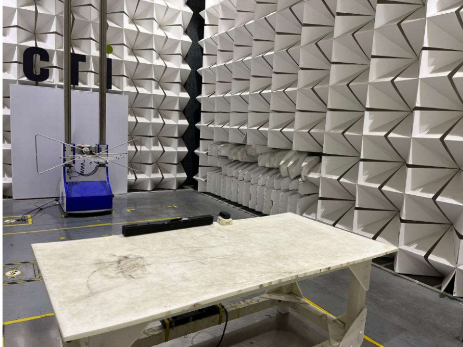
Radiated spurious emission Test Setup-1(Below 1GHz)
