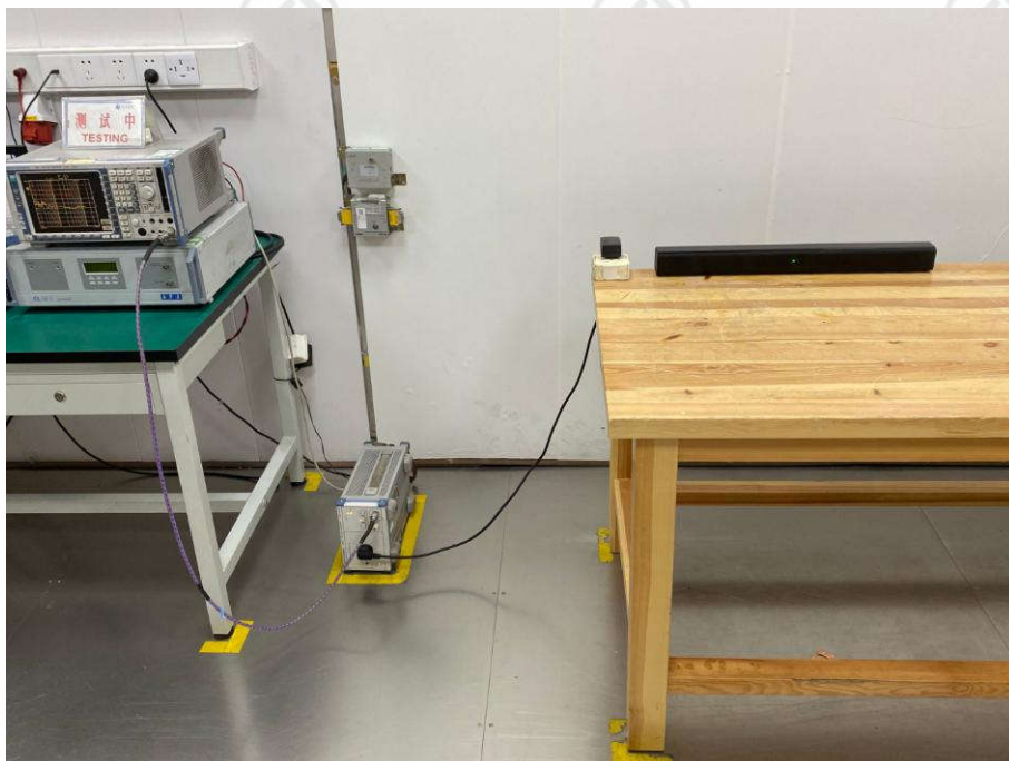
AC Power Line Conducted Emission
