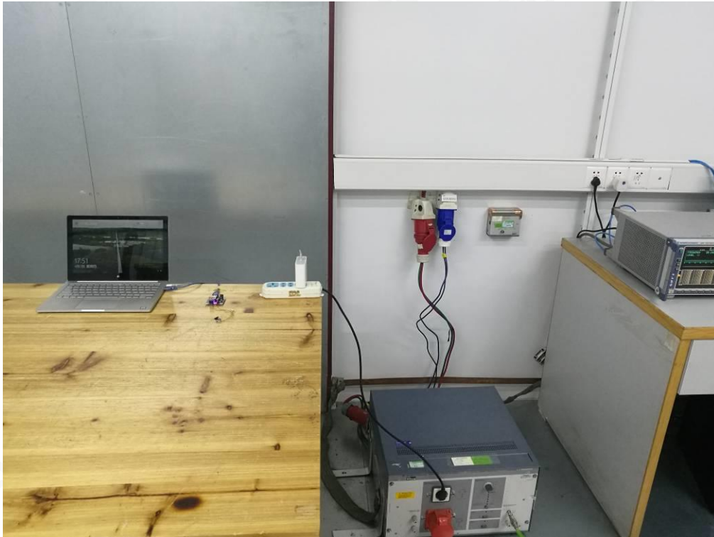
RADIATED EMISSION TEST SETUP BELOW 1GHZ
