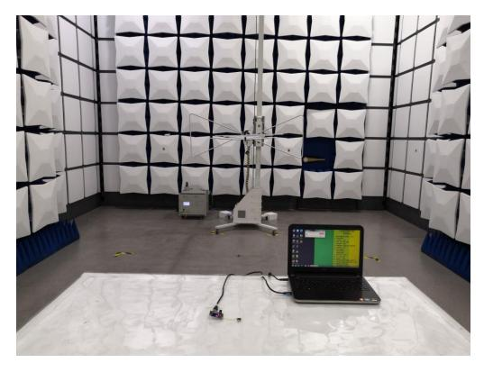
FCC RADIATED EMISSION TEST SETUP ABOVE 1GHZ
