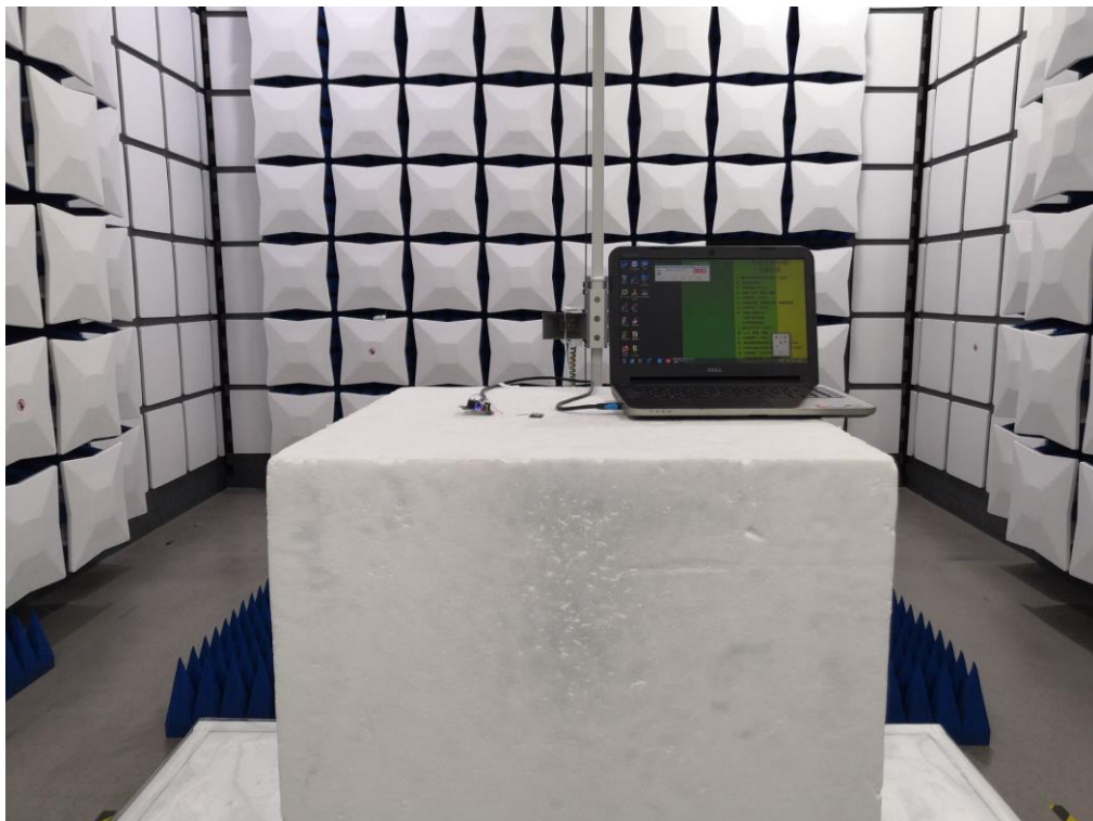
FCC RADIATED EMISSION TEST SETUP ABOVE 1GHZ
